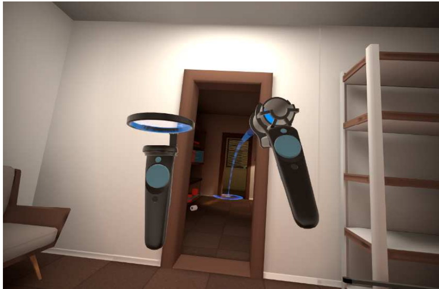
Figure 10.9: A virtual “laser pointer” that follows a parabolic arc so that a destination for teleportation can be easily specified as a point on the floor. (Image from the Budget Cuts game on the HTC Vive platform.)
