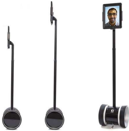
Figure 13.9: The Double telepresence robot is a screen and camera on a stick. The robot costs around $2500, and the screen is a tablet, such as an iPad. The height can even be adjusted remotely so that the person may appear to be sitting or standing.
