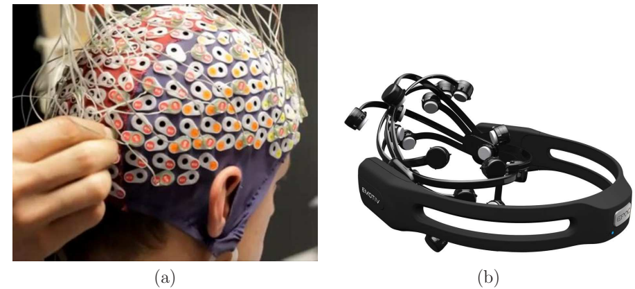
Figure 13.11: EEG systems place electrodes around the skull: (a) A skull cap that allows up to a few dozen signals to be measured. (b) Emotive wireless EEG device.
